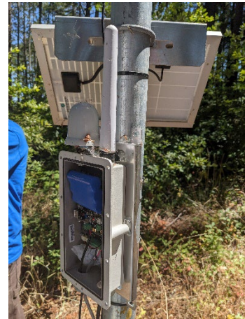
Figure 2. Pole with solar panel, antenna, and data logger for receiving and telemetering data.
